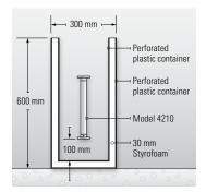
"No stress-strain" enclosure using the Model 4210.
