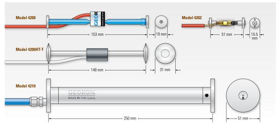
Dimensions of the 4200 Series Strain Gauges.
